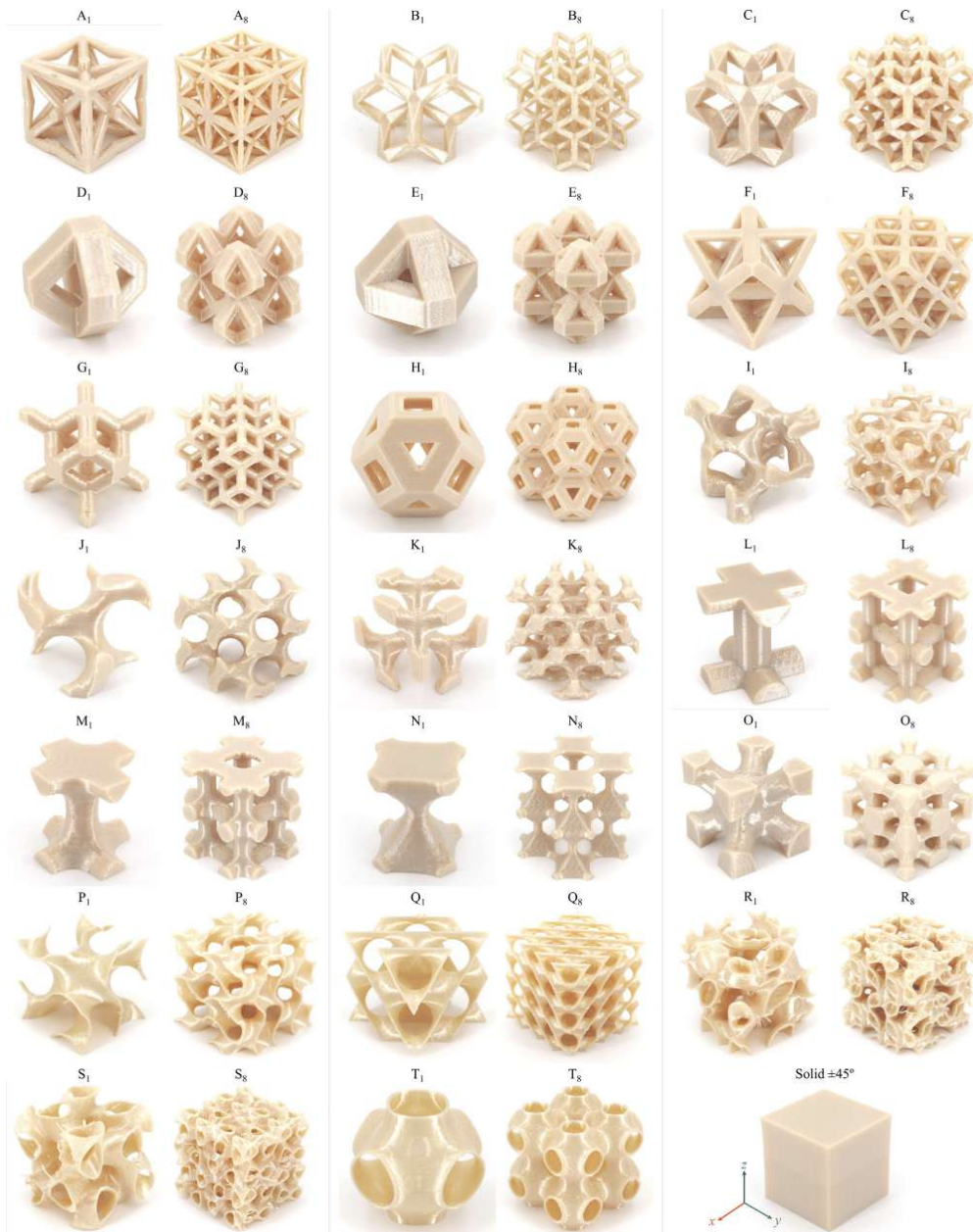
Fig. 1. Unit-cells (Specimen ID 1 ) and eight-cells (Specimen ID 8 ) samples of the three-dimensional patterns manufactured with FFF (see Table 1).
