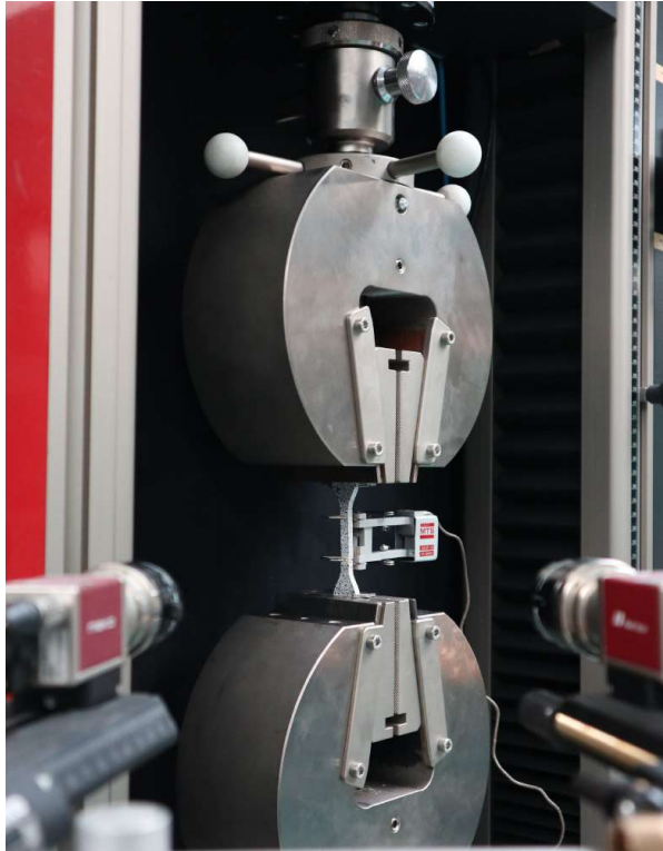
Figure 3.4: Experimental setup for ASTM D638 tensile test standard with DIC equipment.
