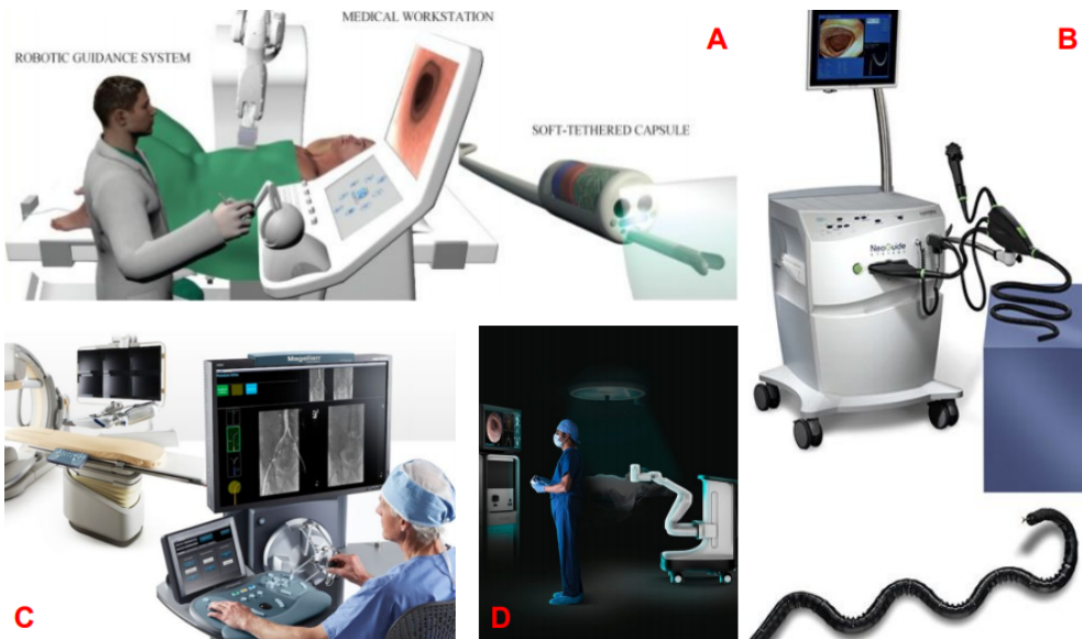
Figure 1.5. Examples of robotic endoscopic devices. A: Endeo platform, magnetic driven colonoscopy capsule [16]; B: The Neo guide multi-articulated snake-like endoscope for colonoscopy [12]; C: Magellan™ Robotic System flexible endovascular robotic endoscope (formerly Hansen Medical Inc. (Mountain View, CA, USA), acquired by Auris Health, Inc (Redwood City, CA, USA)); D: Monarch™ Robotic assisted-bronchoscopy device by Auris Health, Inc (Redwood City, CA, USA) [18].
