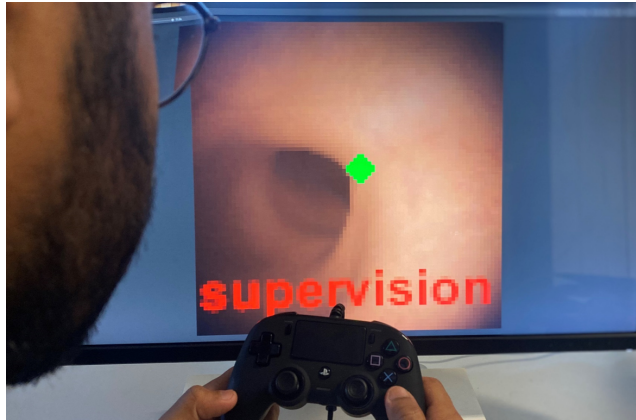
Figure 9.5. Manual supervision through a videogame joystick while navigating by autonomous control strategies. The term supervision is printed on the screen, indicating the switch to teleoperated control. When the endoscope is oriented towards the lumen (green point), the user can give back the control to the autonomous agent. A low-resolution (128x128 pixels) image is displayed to facilitate interpretability of machine decisions, however users have the option to change to high resolution (1024x1024 pixel) display.
