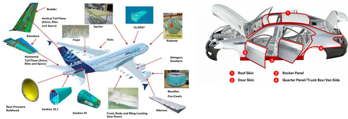
Figure 1-1: example of bonded parts in Airbus A380 (left) and a car (right) [4], [5]
