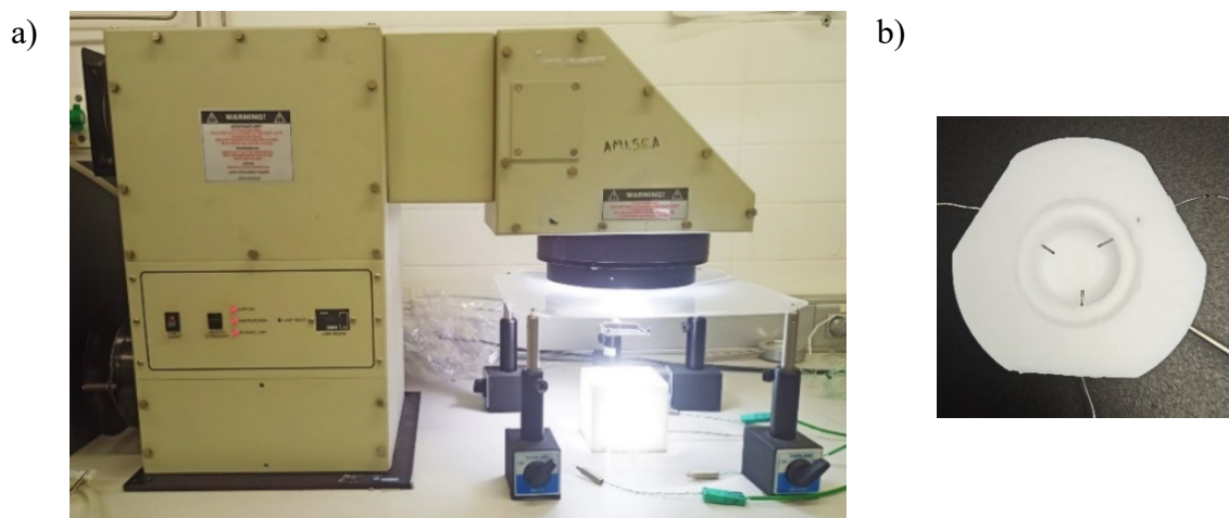
Figure 4.3. Solar simulator PTE a) experimental setup and b) custom-made sample holder.
