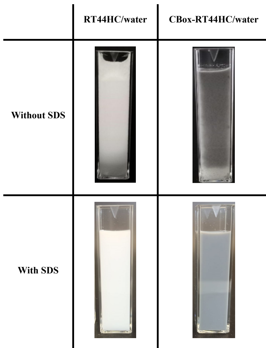
Figure 4.6. Images of RT44HC/water and CBox-RT44HC/water emulsions without and with SDS surfactant 3 days after fabrication.
