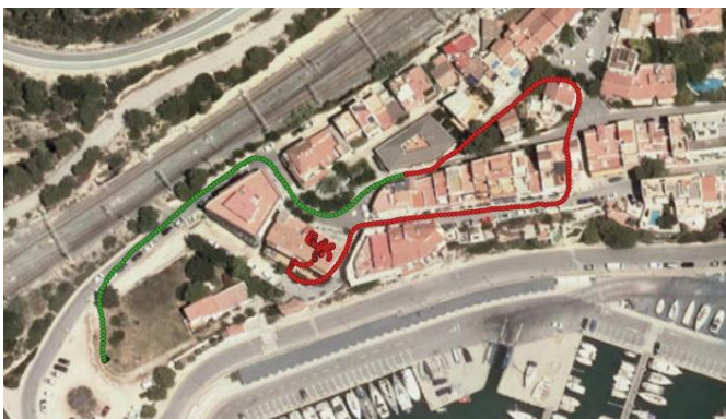
Figure 41. Estimated “Garraf -Town” trajectory. Green dots indicate positions provided by the GNSS while red dots are the ones provided by camera-based tracking system.
