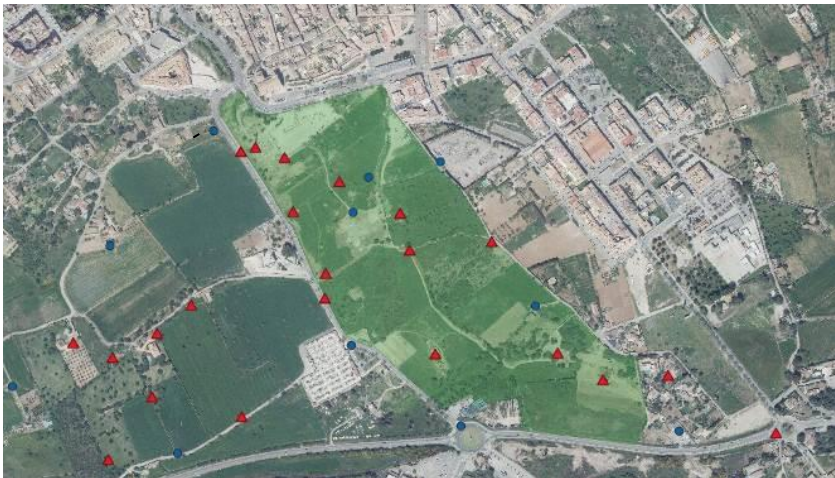
Figure 30. Distribution of ground control (blue dots) and check points (red triangles) around the Roman city of Pollentia (green area) and nearby fields.
