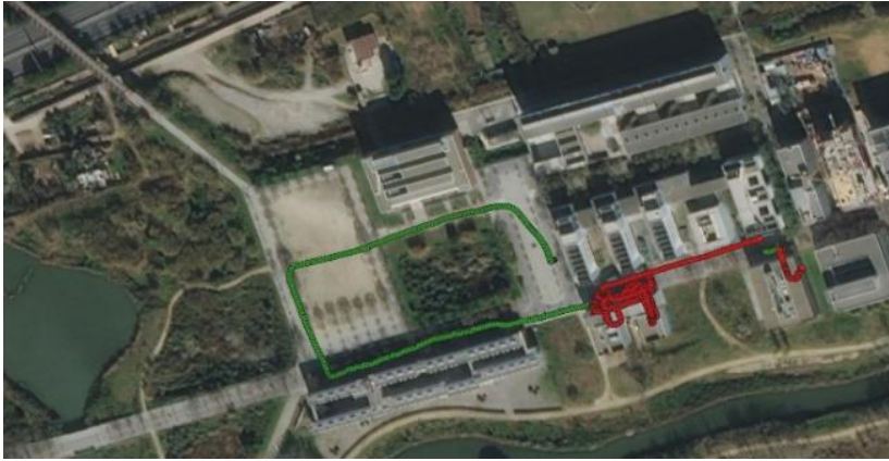
Figure 43. Estimated “PMT-Buildings” trajectory. Green dots indicate positions provided by the GNSS while red dots are the ones provided by camera-based tracking system.
