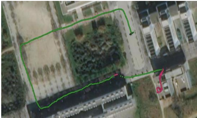
Figure 42. Estimated “CTTC-LAB” trajectory. Green dots indicate positions provided by the GNSS while red dots are the ones provided by camera-based tracking system.
