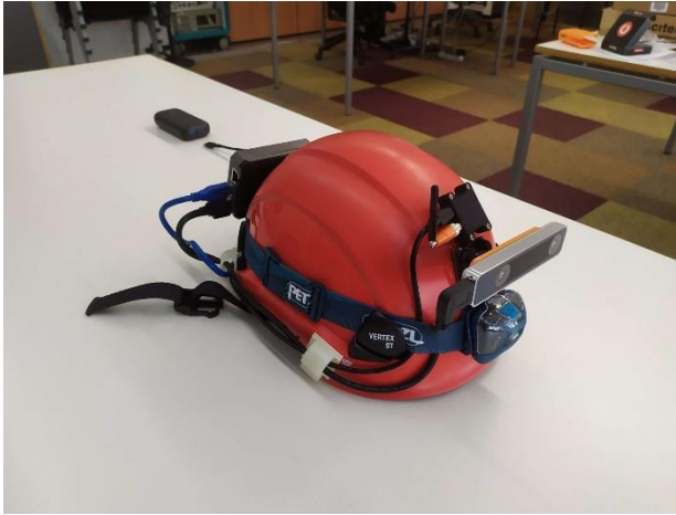
Figure 35. IOPES positioning system mounted on a Helmet.
