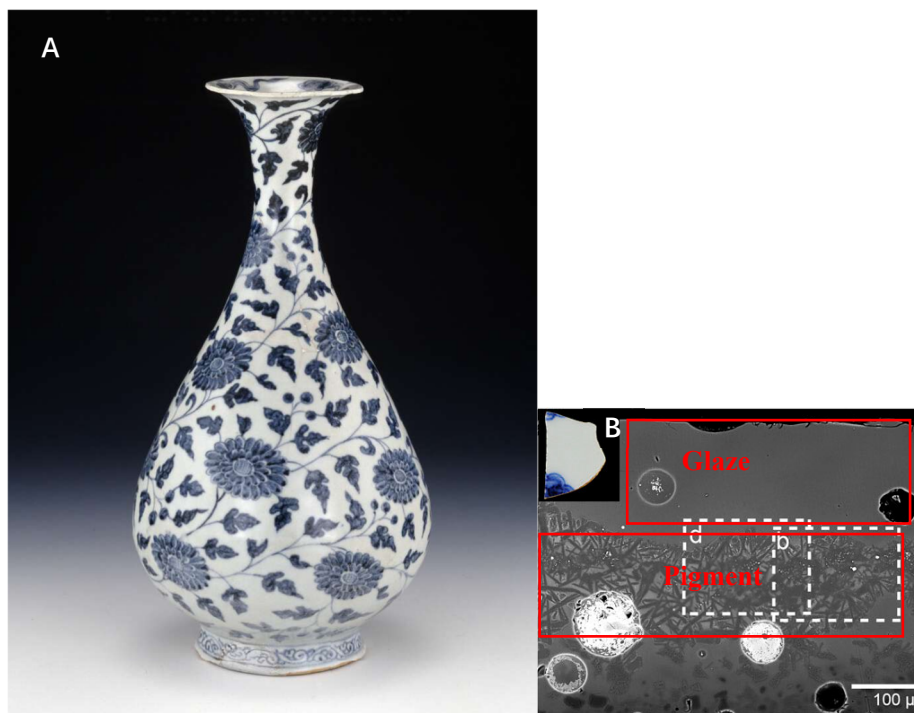
Figure 5.7. (A) White and blue porcelain, Yuan dynasty (c. 1271-1368), The British Museum, https://www.britishmuseum.org/collection/object/A_1924-0114-1 ; (B) One example of the cross-section image of Xuande (1426-1435) imperial blue-and-white porcelain in backscattering mode. (Jiang 2019)
