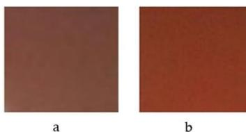
**Figure 6.** Color development of pigments obtained by coprecipitation synthesis with 5% *w/w* CaF<sub>2</sub> (a) and 6% *w/w* (NaF + MgF<sub>2</sub> + Li<sub>2</sub>CO<sub>3</sub>) pigment (b) Y<sub>0.98</sub>Al<sub>0.98</sub>Cr<sub>0.04</sub>O<sub>3</sub> fired at 1400 °C.
