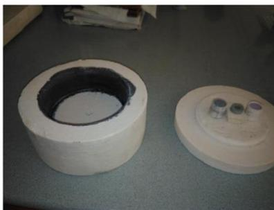
Figure 1. Capsule for a microwave kiln painted with SiC.
