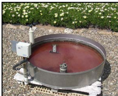
Figure 4.20. An evaporimeter at the experimental water treatment plant in Carrión de los Céspedes (Andalusia).
