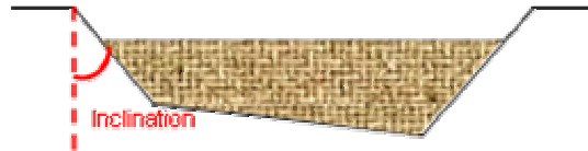
Figure A1.6. Diagram to show the concept of the exterior inclination in the HSCW cells. The red lines show the slope.
