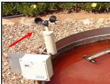
Figure 4.22. The red arrow shows the anemometer located on the evaporimeter at the experimental water treatment plant in Carrión de los Céspedes (Andalusia).
