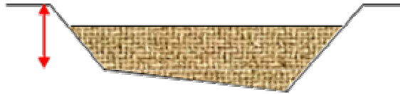
Figure A1.7 Diagram to show the concept of the depth of an HSCW. The red arrow shows the depth.
