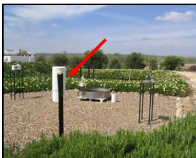
Figure 4.21. Pluviometer at the experimental water treatment plant in Carrión de los Céspedes (Andalusia).
