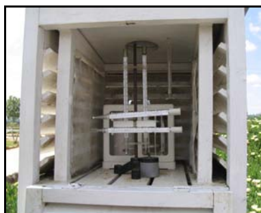
Figure 4.19. Detail of a meteorological station in the experimental water treatment plant in Carrión de los Céspedes (Andalusia). This meteorological station houses a thermometer and a thermohygrometer.
