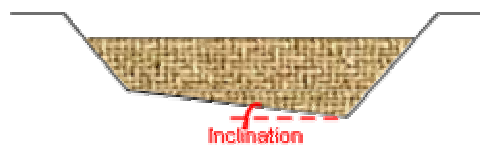
Figure A1.5. Diagram to show the concept of the inclination in the base of the HSCW cells. The red lines show the slope.
