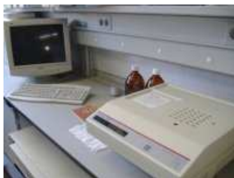
Figura 7. Microtox ® Model 500 Analyser (SDI, USA)
