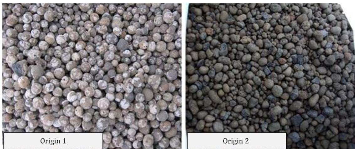
Figure 9 – Lightweight aggregates from different origins.
