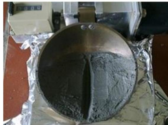
Figure 7 – Grooving the mortar sample before the Atterberg liquid limit test.
