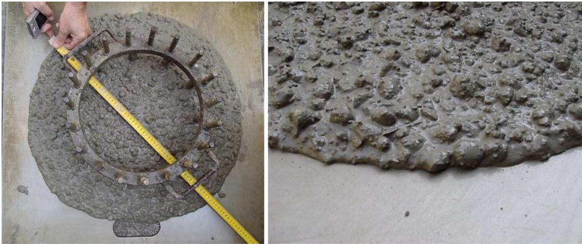
Figure 10 – Slump flow test with the Japanese ring and the edge of concrete, concrete P<sub>9</sub>.
