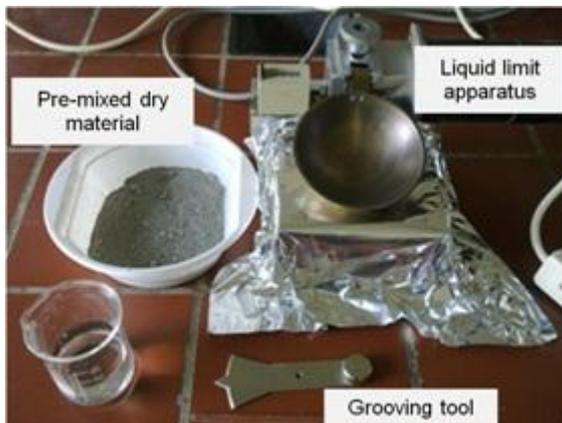
Figure 6 – Materials and equipment used for the Atterberg liquid limit test.
