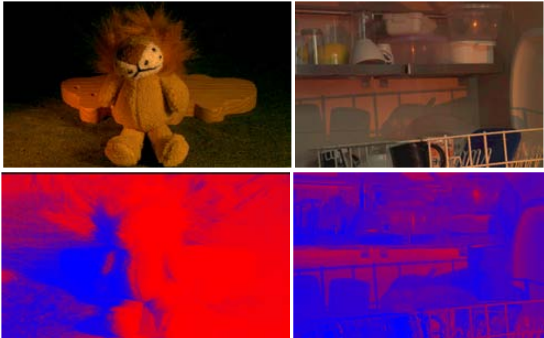
Figure 4.1: Sample images from our database. The bottom row shows the relative influence of the two incident illuminants color-coded in blue and red.
