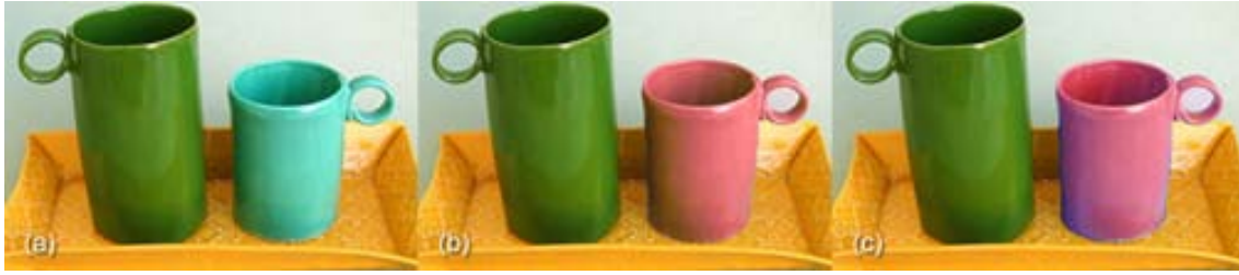
Figure 3.8: Comparing the MIDR method performance with a professional photo-editor: (a) Original image (containing complex interreflection); (b) Recoloring result by MIDR (the secondary illuminant, green interreflection, has been preserved); (c) Recoloring result using the hue-saturation shift method (the green interreflection is wrongfully changed to blue).
