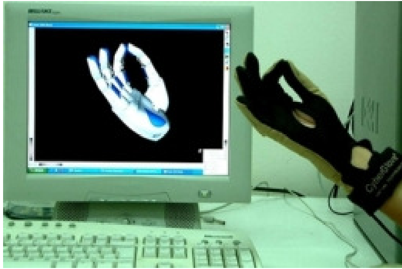
Figure 6.2: A human hand with a sensorized glove connected to the mechanical hand simulator.
