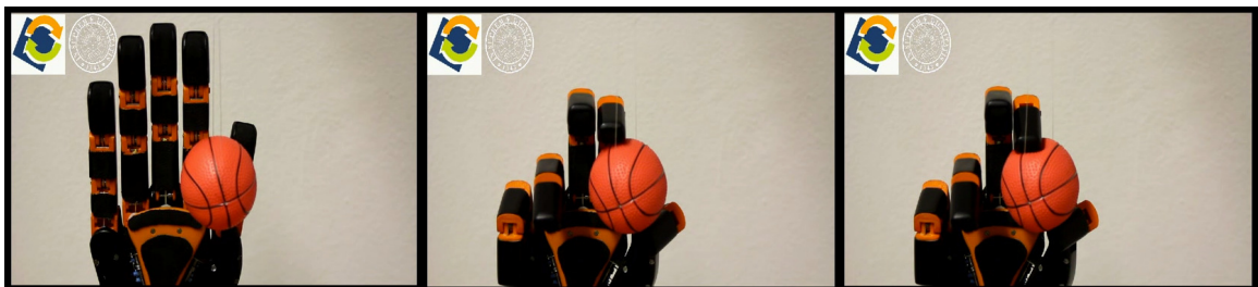
Figure 5.6: A solution obtained and implemented on THE First Hand [8]. The object is placed at the computed position (left). The fingertips make contact at the object surface satisfying the reachability constraint (middle). The fingers perform the squeezing action to firmly hold the object (right).
