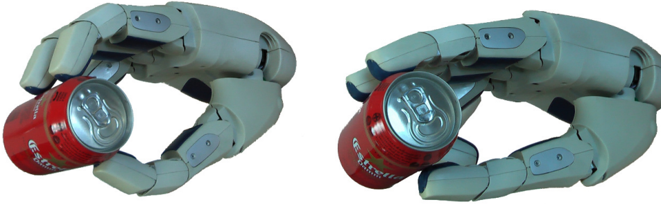
Figure 4.1: Two grasps of a can for drink service. While both grasps are force-closed and manipulable, the grasp on the left is preferable. The fingers are almost fully extended in the grasp on the right, limiting the possibility to move the can in one direction.
