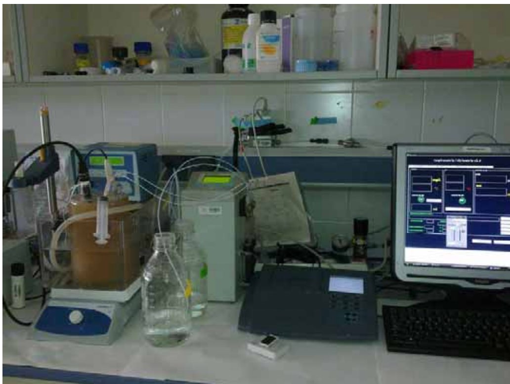
Figure 5.2. Experimental set-up of the LFS Respirometer-titrimeter used for batch experiments.
