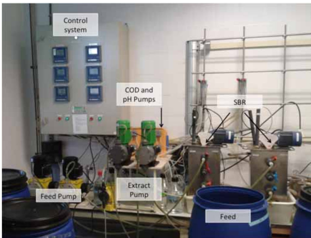
Figure 3.1. EBPR-SBRs Pilot Plant.
