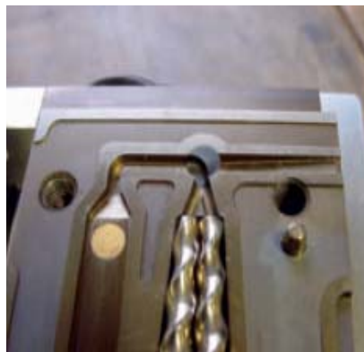
Figura 15: Extrusor Haake MiniLab, detall del doble vis-sens-fi
