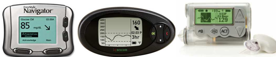
Figure 2.10: Current CGM devices used in home monitoring: the Abbott FreeStyle Navigator ® continuous glucose monitoring system, the DexCom SEVEN ® , and the Medtronic MiniMed Paradigm ® REAL-Time insulin pump and continuous glucose monitoring system.
