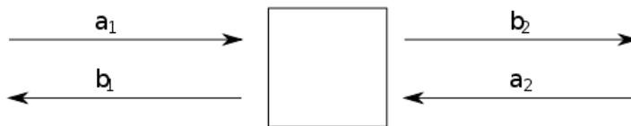
Figure 5.14: S-parameters incident and reflected waves representation.
