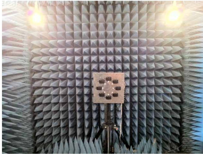
Figure 5.85: Antenna array and front-end calibration setup in an anechoic chamber.
