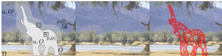
Figure 1: Inpainting problem. On the left: the original image. In the center: the result of one of the exemplar-based inpainting scheme derived from the variational framework presented in this thesis. On the right: the red curves show the boundaries between regions that have been copied from a corresponding region in O^c .
