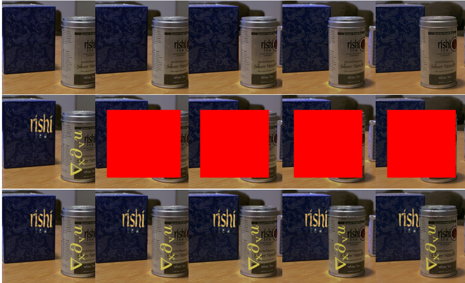
Figure 13.5: The first row shows the original sequence. A box and a cylindrical can are being filmed while the camera moves. The second row shows the input sequence after editing the first frame and where the editing domain has been marked in red. The third row shows the output after minimizing (13.1). From left to right, the frames shown correspond to t = 0, 2, 5, 9 and 12 respectively.
