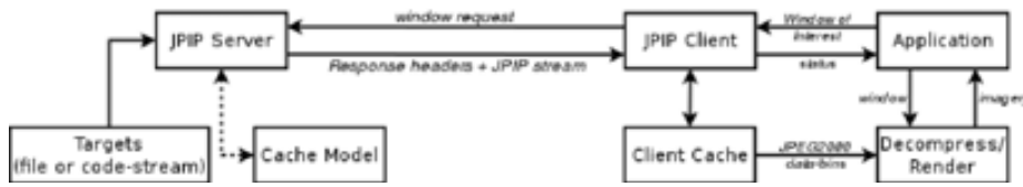
Figure 1.1: JPIP protocol architecture. The server side is composed of a JPIP Server, the core of the server, a Cache Model to keep track of data sent to clients, and the images to be served. The client side is composed of the end-user application, the JPIP Client that carries out the communication with the server, a Client Cache where data received are stored, and the image decompressor.
