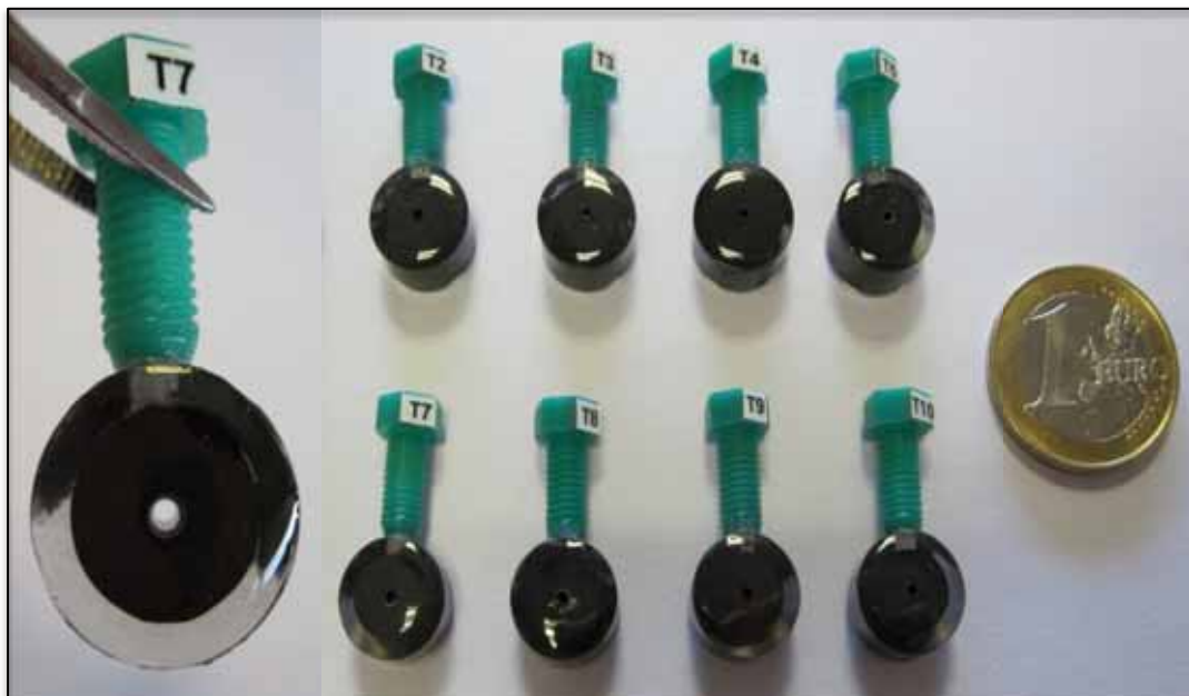
Figure 4.9 Images of constructed tubular electrodes of polymeric liquid membrane for \text{SO}_4^{2-} analysis
