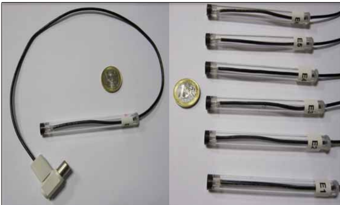
Figure 4.11 Images of constructed conventional electrodes of polymeric liquid membrane for \text{SO}_4^{2-} batch measure
