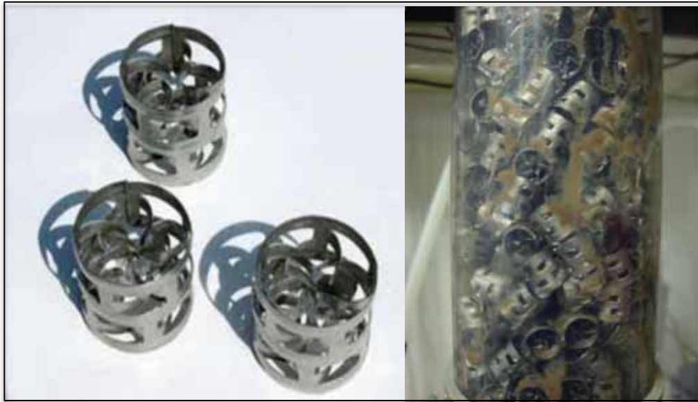
Figure 4.3 Images of packing material before and after BTF packing
