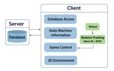
Figure 6.6: The integration of Kinect into LISSA system
