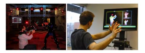
Figure 6.1: Optical-based motion tracking system with markers (left) and marker-free (right)
