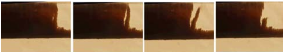
Figure 5.5. Magnetic plug stability when the flow rate is increased up to 200 \mu\text{L min}^{-1} .
