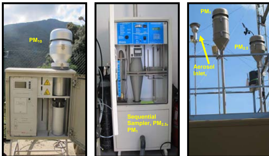
Figure 2.5. High-volume sampler MCV-CAV-A/M-S sequential high volume sampler (left) with an MCV inlet, DIGITEL DH-80 sequential high volume sampler inside the cabin (centre) and PM DIGITEL inlets for \text{PM}_1 and \text{PM}_{2.5} protruding above the cabin roof (right). The custom designed aerosol inlet (Thermo, \text{PM}_{10} ) is also shown (right).
