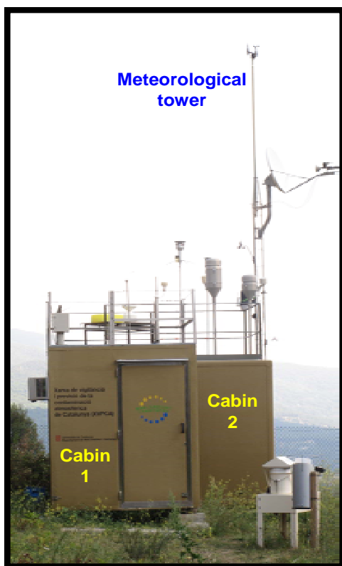
Figure 2.2. Climate controlled cabins at the MSY station containing aerosol monitoring equipment.
