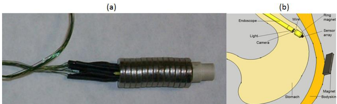
Figure 7. Picture of the fabricated array with the magnet rings around (a). Scheme of the endoscopic insertion and stabilization of the array inside the stomach (b).
