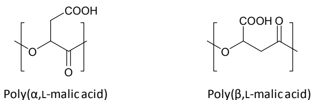
Figure 2.4. Chemical structure of poly (malic acid) stereoisomers.
