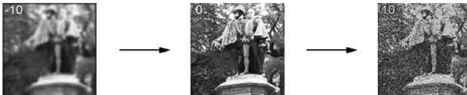
Fig. 3.3: Test image set for illustrating the anisotropy measure. Blur decreases from -10 to 0 and noise increases from 0 to 10 . The central image is the original source image (from Gabarda & Cristóbal (2007)).
