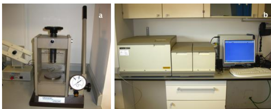
Figure 4.2. Pictures of the compressor to create the pellets (a) and FTIR Perkin-Elmer 2000 spectrophotometer (b).
