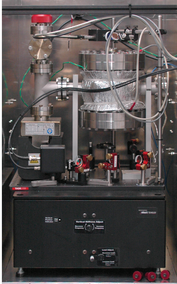
Figure 4.8.: Picture of the vacuum chamber containing the high-finesse cavity. The whole set-up is resting on a passive vibration-damping platform and is surrounded by a temperature-stabilized aluminum box.
