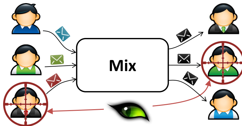
Figure 2.3: Many of the current ACSs are built upon the idea of Chaum’s mix. Essentially, a mix can be seen as a black box that forwards messages in such a way that prevents an adversary from linking an outgoing message to its corresponding input message.
