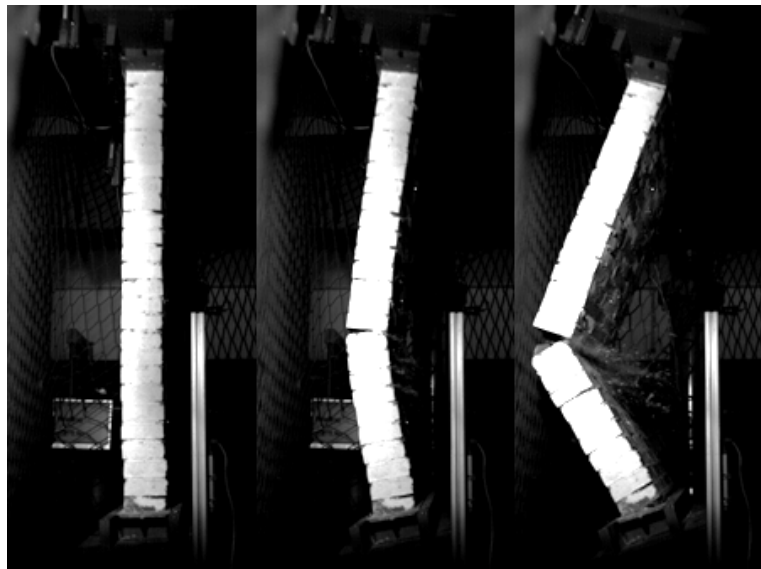
Figure 3.16 Failure mode of wall W#10. Opening of a joint and mechanism formation
