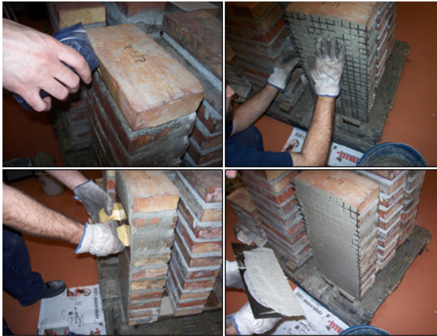
Figure 3.7 TRM application procedure on the brick masonry prisms
