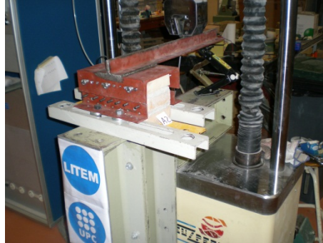
Figure 3.6 Bond wrench test set up for determining the mortar-brick bonding strength
