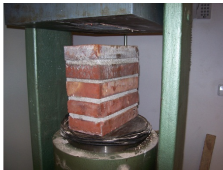
Figure 3.4 Compressive strength test of a brick masonry prism from the D series
