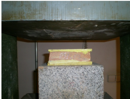
Figure 3.3 Compressive strength test on a half brick
