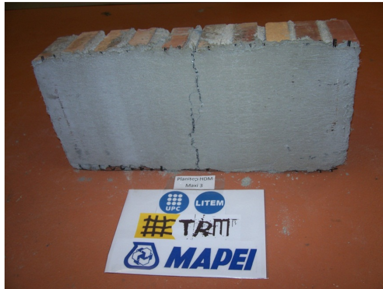
Figure A1. 50. Mid-span cracking. Failure mode of the sample M3
