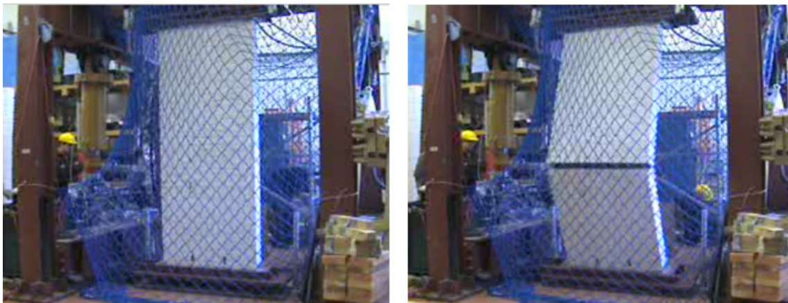
Figure A1.131 Wall W#6 at the beginning of the test (left) and failing (right)
