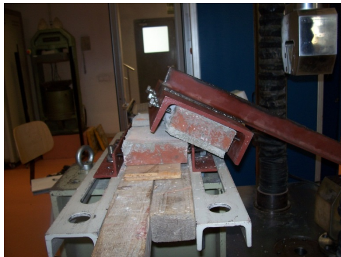
Figure A1. 37 Failure mode of the mortar-brick adherence tests
