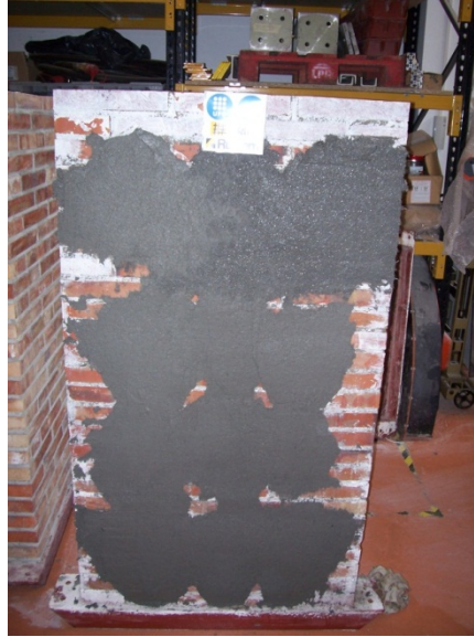
Figure A1. 87 Connectors bonding on the non-strengthened face of wall W#29.
