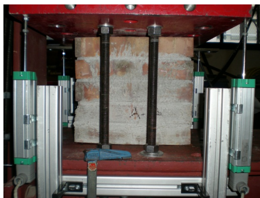
Figure A1. 33 Set up for the test to obtain the modulus of linear deformation of brickwork
