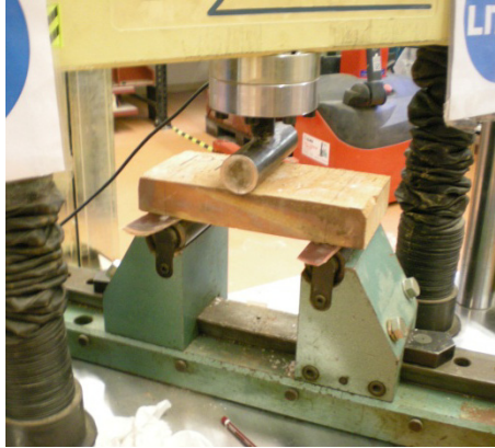
Figure A1. 26 Brick flexural strength test set up
