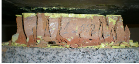
Figure A1. 29 Typical crushing failure of a uniformly compressed brick
