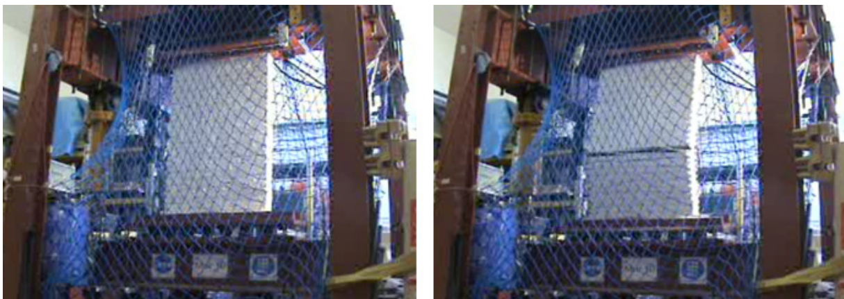
Figure A1. 147 Wall W#10 at the beginning of the test (left) and failing (right)
