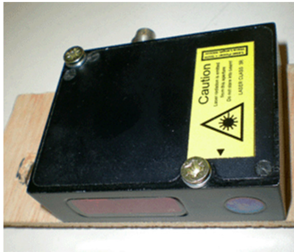
Figure A1. 95 Riftek RF-603 laser position sensor
