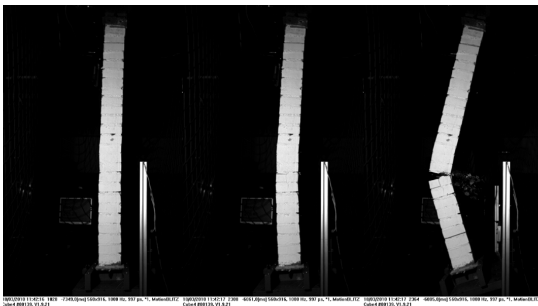
Figure A1. 174 Failure of the wall W#16. Opening of a horizontal joint at 1/3 of the height.
