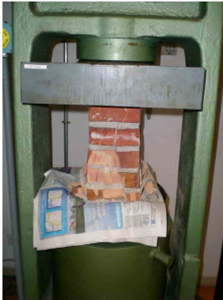
Figure A1. 34 Crushing failure of a brickwork prism under the compressive strength test
