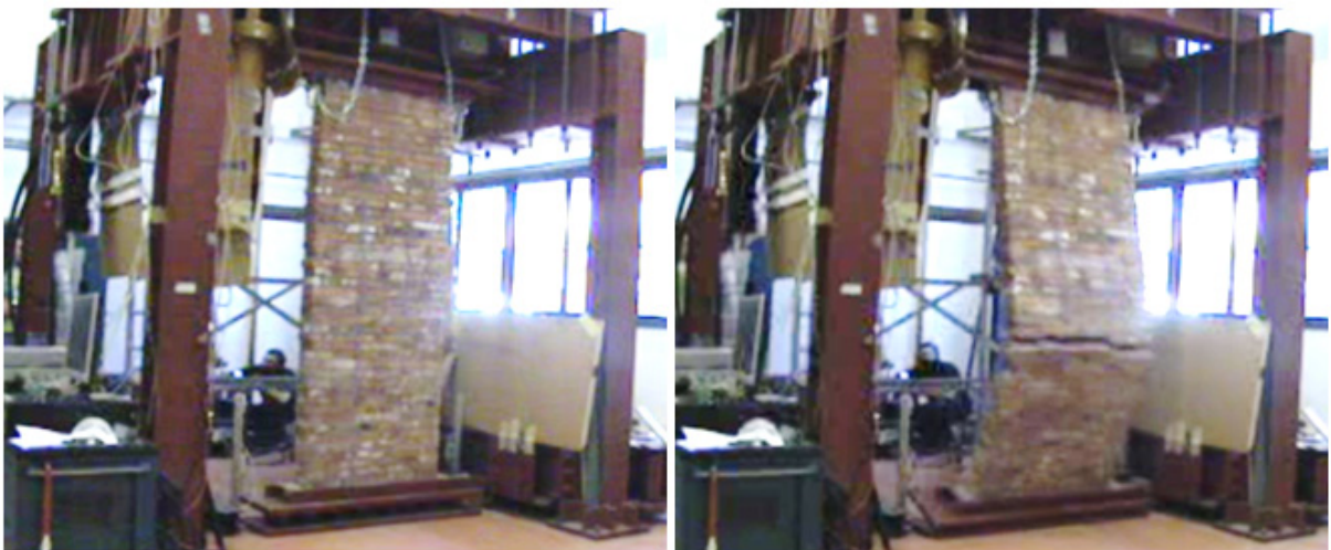
Figure A1. 110 Wall W#1 at the beginning of the test (left) and failing (right)
