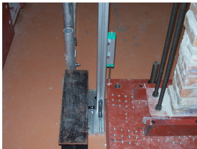
Figure A1. 107 Potentiometer for the measure of the rotation of the lower hinge valid for H series walls
