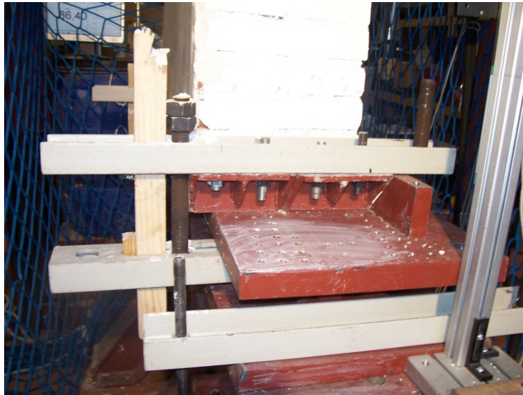
Figure A1. 92. Wall-hinge connection system specially used in wall W#17 (T series)
