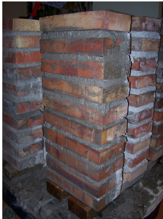
Figure A1. 43. View of a wetted sample ready to receive the first mortar layer
