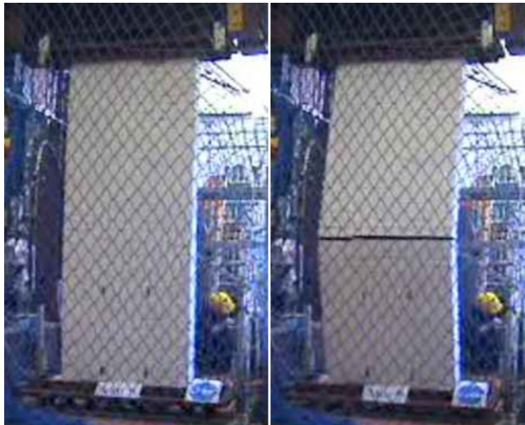
Figure A1. 143 Wall W#9 at the beginning of the test (left) and failing (right)
