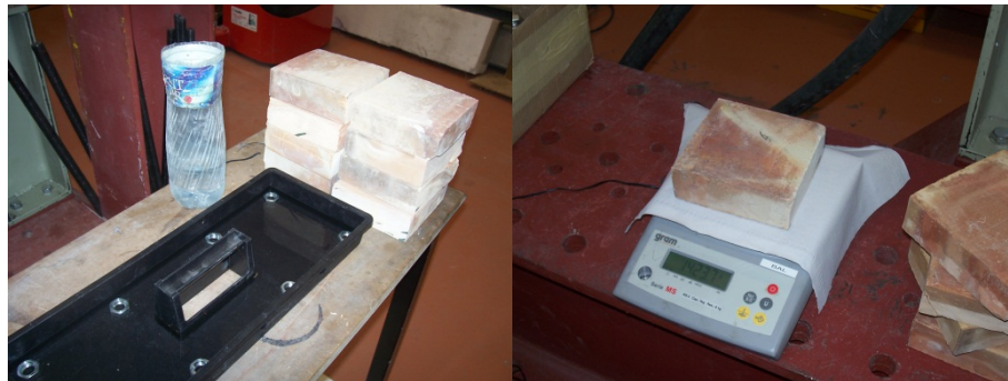
Figure A1. 30 Water absorption test set up and scales used
