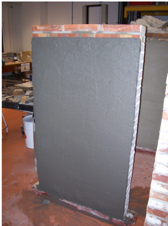
Figure A1. 86 Final state of a TRM strengthened wall with 6 connectors (W#28)
