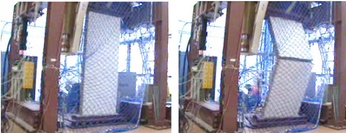
Figure A1. 114 Wall W#2 at the beginning of the test (left) and failing (right)
