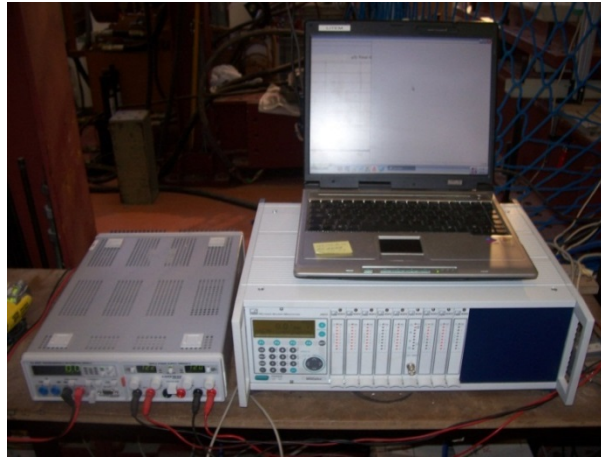
Figure A1. 101 Voltage supply source for lasers (left), MGCPlus data acquirer (down) and controlling laptop (up)
