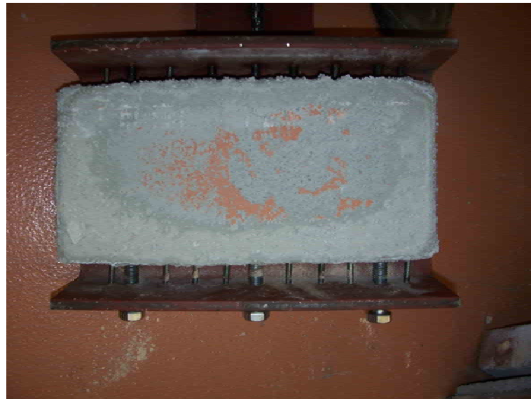
Figure A1. 40 Peeling effect in mortar-brick adherence tests
