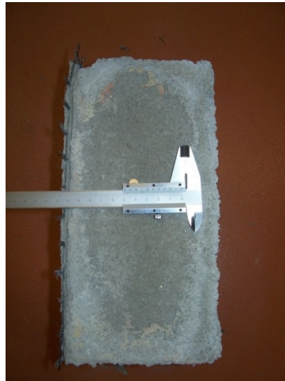
Figure A1. 49 Measuring the fibre grid position, the mortar thickness and the number of fibre rows contained in the mid-span section of sample M2
