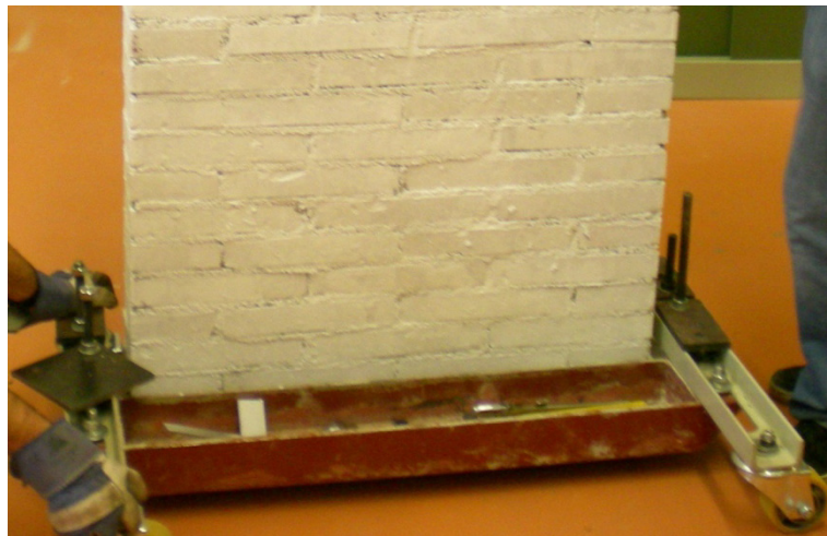
Figure A1. 68 Elevation and displacement tool. Wall W#10.
