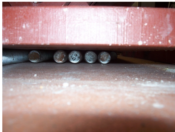
Figure A1. 71 Using rods to move walls of H and F series
