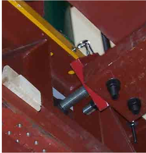
Figure A1. 89 Tool (steel plate and bar) to keep the vertical alignment of the distribution beam in test W#1
