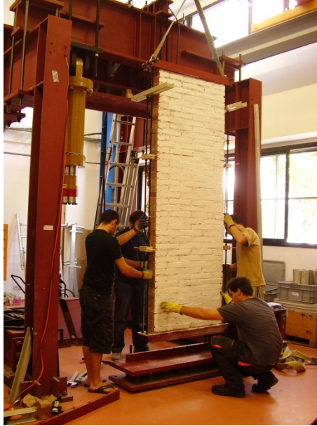
Figure A1. 70 Moving wall W#2 with the crane and leaving it on the lower hinge.
