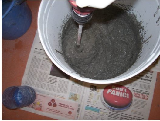
Figure A1. 44. Mixing procedure of mortar XMesh M25 for strengthening samples X1, X2 and X3
