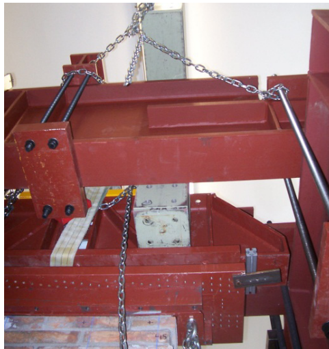
Figure A1. 90 Upper area of the test setup for wall W#1. The distribution beam was held by chains and vertically aligned with only one steel pillar.
