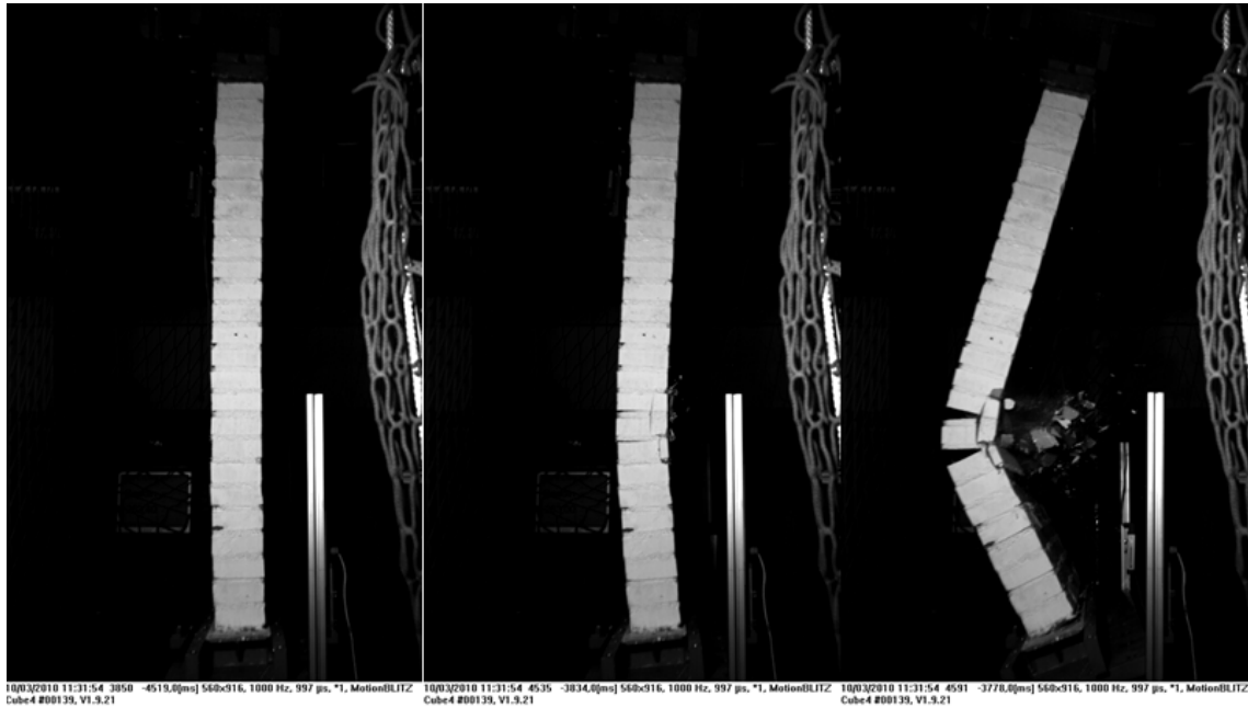
Figure A1. 166 Failure of the wall W#14. Crushing at compression side and opening of a horizontal joint
