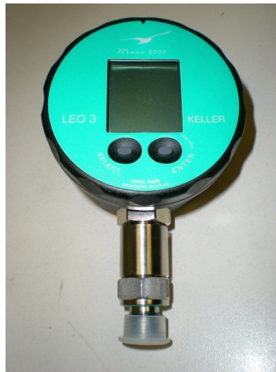
Figure A1. 93 Keller LEO-3 pressure sensor
