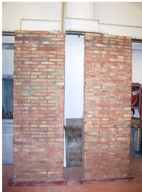
Figure A1. 57 Walls W#4 and W#5 build inside laboratory facilities
