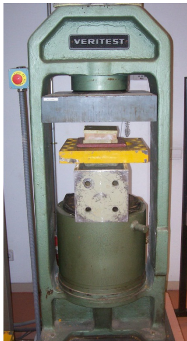
Figure A1. 28 Brick compressive strength test set up
