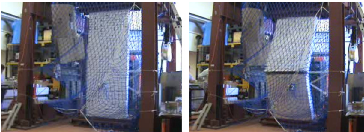
Figure A1. 118 Wall W#3 at the beginning of the test (left) and failing (right)
