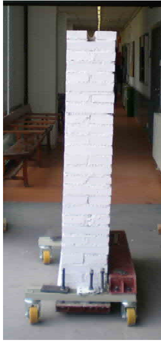
Figure A1. 67 Displacement of the wall W#17
