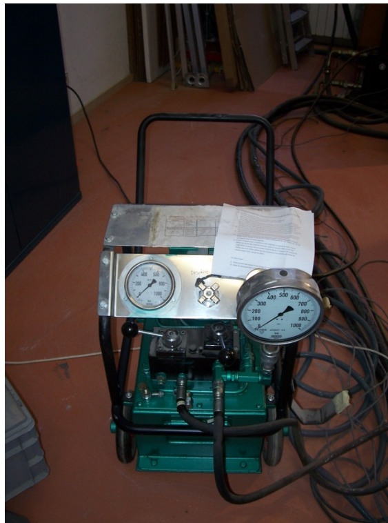
Figure A1. 102 1000bar pump for providing the oil pressure needed by the jack
