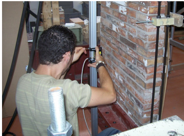
Figure A1. 106 Measuring the geometry of wall W#1
