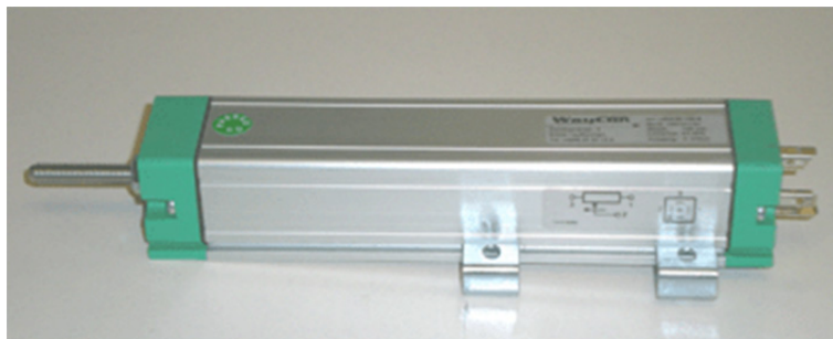
Figure A1. 96 Waycon LRW-100 displacement potentiometric sensor
