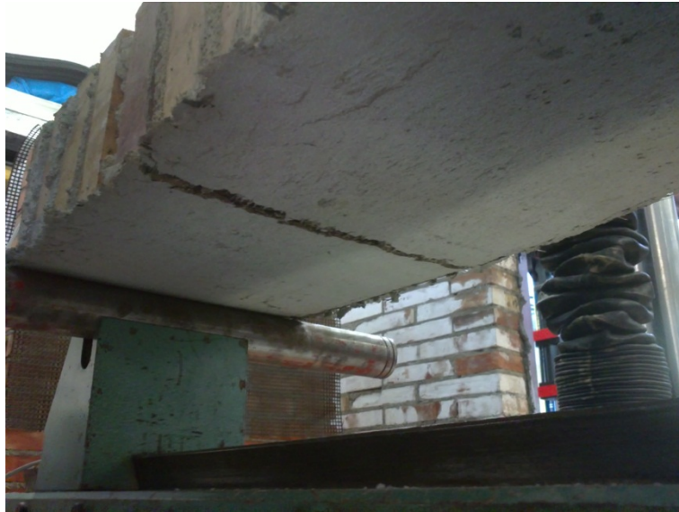
Figure A1. 51 Bending failure of the sample R2. One big crack in the mid-span breaking the TRM strengthening system
