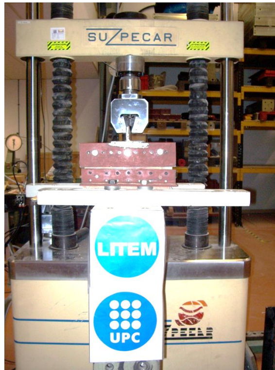
Figure A1. 36 Testing machine and setup for the mortar-brick adherence tests
