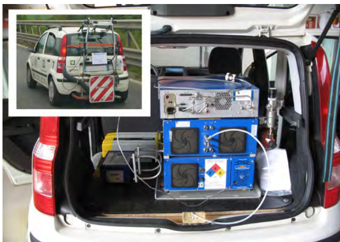
Figure 2.6: Passenger car instrumented with PEMS
