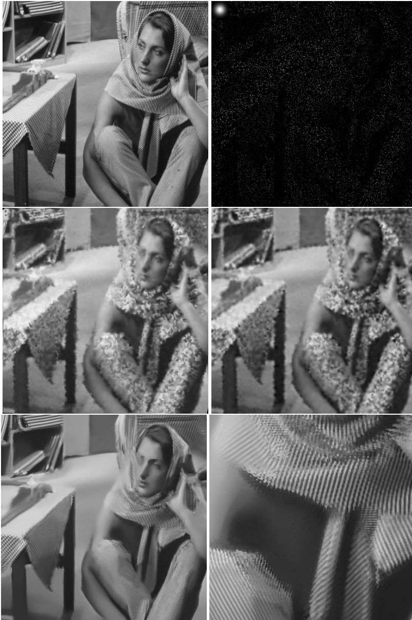
Figure 7.9: Interpolation with lower sampling density. From left to right top to bottom: original image Barbara 512 \times 512 , the available samples 5% of the samples, the result of linear interpolation over the Delaunay triangulation (PSNR 20.1), results of the Laplacian interpolation (PSNR 19.9) and the output of algorithm O with h = 100 (PSNR 22.8).
