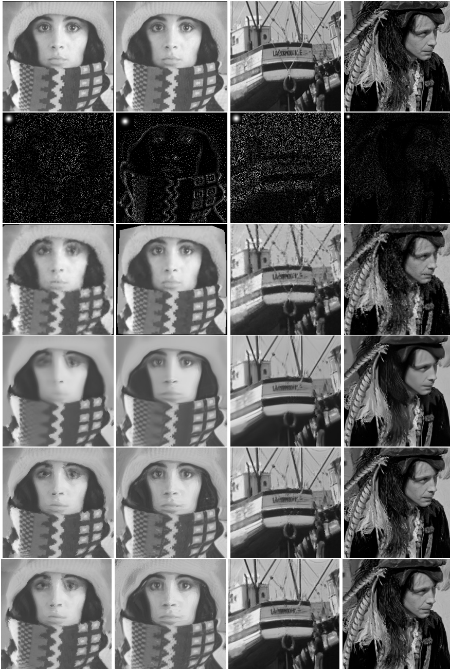
Figure 7.7: Sparse sampling interpolation. 1st row: original images. 2nd row: input data with sample densities of 10%, 10% dithered [BBW08], 20% and 9%. 3rd row: linear interpolation over the Delaunay triangulation of the samples; PSNRs: 25.8, 30.6 (not considering the black frame), 25.0 and 22.74. 4th row: results of method AB with h = 100 ; PSNRs: 22.5, 22.7, 25.5 and 22.79. 5th row: results of AB with h \rightarrow 0 ; PSNRs: 22.6, 23.0, 25.5 and 22.56. 6th row: results of the method O with h \rightarrow 0 ; PSNRs: 22.6, 21.7, 25.1 and 22.69. (Details can be better appreciated by zooming on a computer screen)
