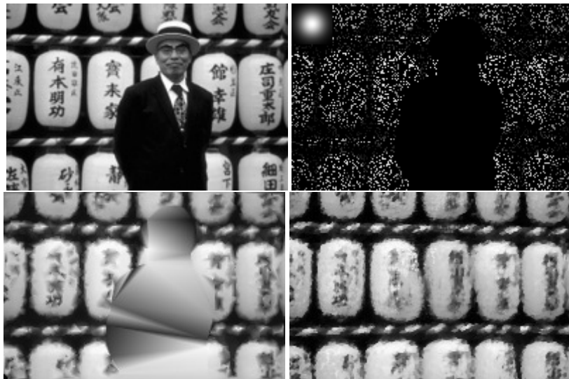
Figure 7.8: Inpainting experiment. From left to right top to bottom: the original image Mitama Matsuri 200 \times 113 , the available samples (the sampling density outside the hole is 20% yielding a global sampling density of 14%), the result of linear interpolation over the Delaunay triangulation and the result of algorithm B . The algorithm makes no distinction between the hole and the sampled regions.
