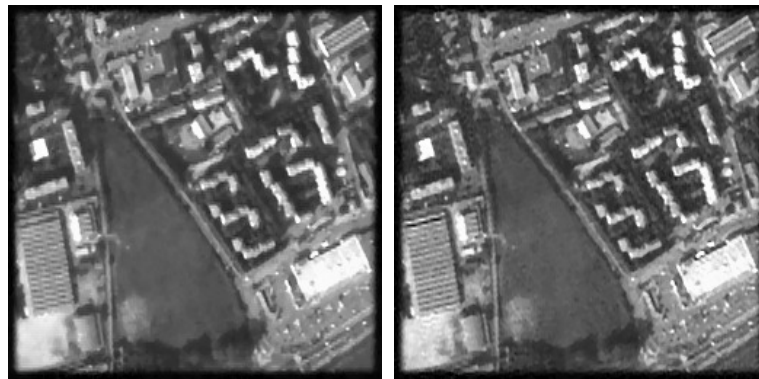
(a) Fusion using the supermode projector. ( MSE = 19.7 ) (b) Fusion using the spectral projector computed with the generalized supermode. ( MSE = 21.0 )
