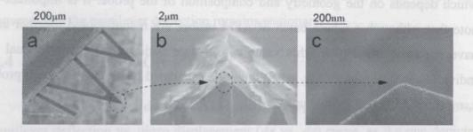
Fig. 5. a)  $Si_3N_4$  triangular and rectangular cantilevers mounted on the same chip. b) Zoom of the tip. c) Zoom of the tip apex, with a R around 50nm.
