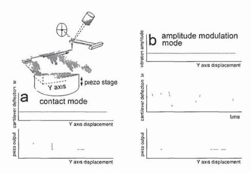
Fig. 8. The two classic modes of topographic AFM operation: contact and amplitude modulation mode. a) In contact mode, the feedback loop keeps  $\Delta x$  constant while the piezo output responds to the sample topography. b) In amplitude modulation mode, the cantilever oscillates at its resonance frequency. The feedback loop maintains the vibration amplitude constant, while the piezo response is the topographic signal.
