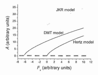
Fig. 17. Dependence between A and  $F_{\nu}$  for the most common contact mechanics models: Hertz, JKR and DMT. JKR model predicts the higher contact areas, while hertzian contact cannot be extended to negative  $F_{\nu}$  values, as it does not take into account any adhesive force.
