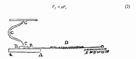
Fig. 2. Amontons' machine designed to perform friction measurements.  $F_f$  between the surfaces A and B are measured by the spring D, while  $F_{\nu}$  is controlled by the spring C, which pushes the slider against the tested surface. As you can see, the design is quite advanced, which implies that Amontons had a clear idea about the meaning of macroscopic friction.
