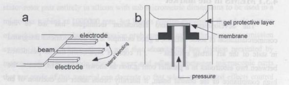
Fig. 21. Examples of commercial MEMS. a) micro-accelerometer. When acceleration changes, the central beam bends laterally, modifying the capacitance of the system. The complete device consists on an array of electrode-beam-electrode units oriented in perpendicular directions and suspended on springs so as to be sensitive to accelerations in all axes. b) Pressure sensor. As pressure changes, a change of resistivity is detected by the piezoresistors placed in the membrane.
