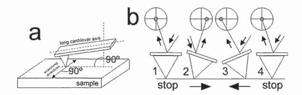
Fig. 12. LFM operation. a) The tip scans the surface perpendicularly to the main cantilever axis. b) Whole friction measurement (friction loop): 1 - the cantilever stands still on the surface. 2 - the tip scans the sample from left to right, creating a cantilever torsion that is detected by the photodetector. 3 - the same process but scanning from right to left. Now the laser spot is in the left side of the photodetector. 4 - end of the loop.
