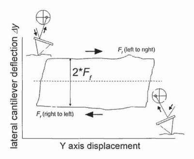
Fig. 13.  $\Delta y$  vs. Y axis displacement while a friction loop is performed. The area of the loop is proportional to the total energy dissipated during the process and  $F_f$  in a certain position is proportional to the half width of the friction loop, as expressed in equation 9.
