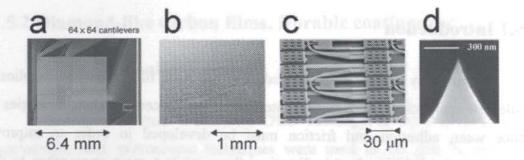
Fig. 23. Millipede® project, devoted to create a high information density write-read device. a) Whole array of 4096 AFM-like probes. b) and c) Zooms of the device, where individual cantilevers can be resolved. d) SEM image of an individual tip apex, used as a writing and reading tool. Images extracted from www. zurich.ibm.com/ st/storage/millipede.html
