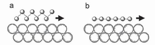
Fig. 3. Phononic friction. a) liquid layer sliding on a solid surface. Due to the low interaction between liquid molecules, it is easy for them to commensurate with the solid substrate and increase  $F_f$ . b) Solid layer sliding on the substrate. The sliding layer cannot keep track with the substrate interatomic distance and slides with low  $F_f$ .
