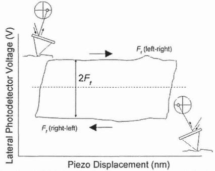
Figure 2. Shape of a typical friction loop. The Y axis represents the lateral photodetector signal as the tip slides on the sample surface. The Y axis can be converted to  $F_l$  if the lateral force constant  $(k_l)$  and the lateral sensitivity  $(S_L)$  of the cantilever are known.
