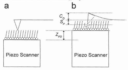
Figure 4. Sample and cantilever deformation as a force curve is performed. a) The tip and the sample are in contact, prior to any cantilever deflection or sample deformation, b) As the Z piezo moves the sample up  $(Z_{PD})$ , the cantilever deflects  $(C_D)$  and the sample is penetrated  $(S_D)$  according to  $Z_{PD} = S_P = C_D$
