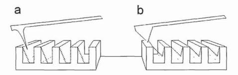
Fig. 6. a) High-aspect ratio tip, suitable for imaging deep trenches. Notice that, although this tip accurately measures the trench depth, it does not track its shape exactly. Consequently, choosing the correct tip for each job is extremely important. b) Low-aspect ratio tip, which measures both an incorrect trench depth and shape. The dotted lines in both figures mark the topographic image recorded by each tip while the solid lines are the real trench shapes.
