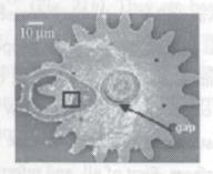
Fig. 20. Micrometric gear showing serious wear problems. Courtesy of Sandia National Laboratories, SUMMiTTM Technologies, webpage; www.mems.sandia.gov.
