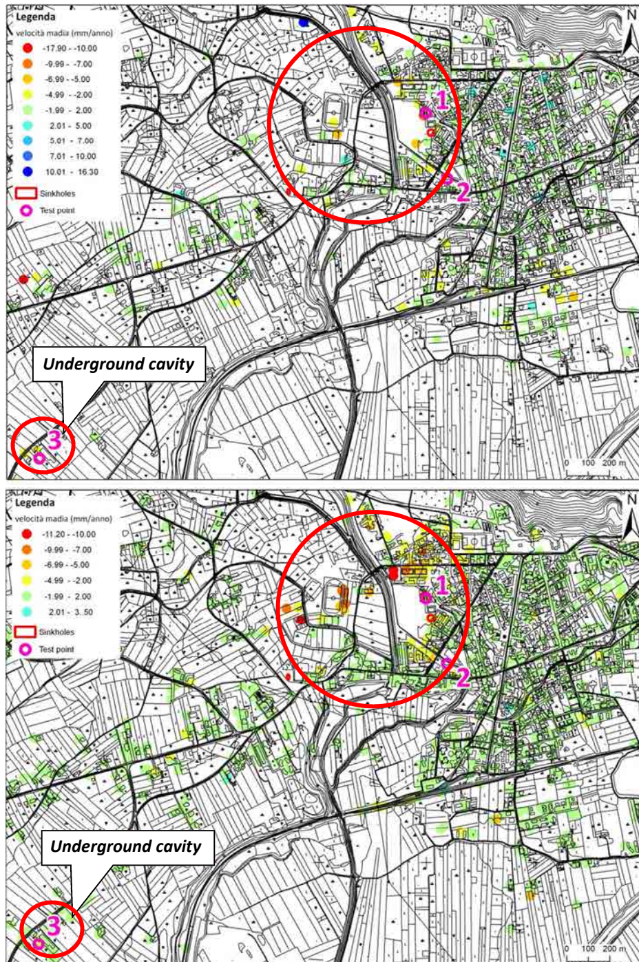
Figure 6.69: CPT processing results (above); PS DInSAR data (below)
