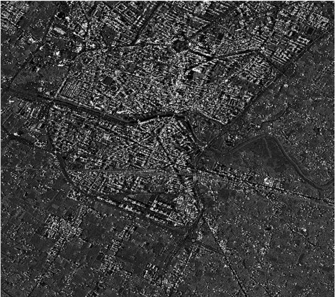
Fig. 4.13: Amplitude high resolution image obtained using 121 available X-band images of Murcia (pixel resolution 1.5x1.9 m)
