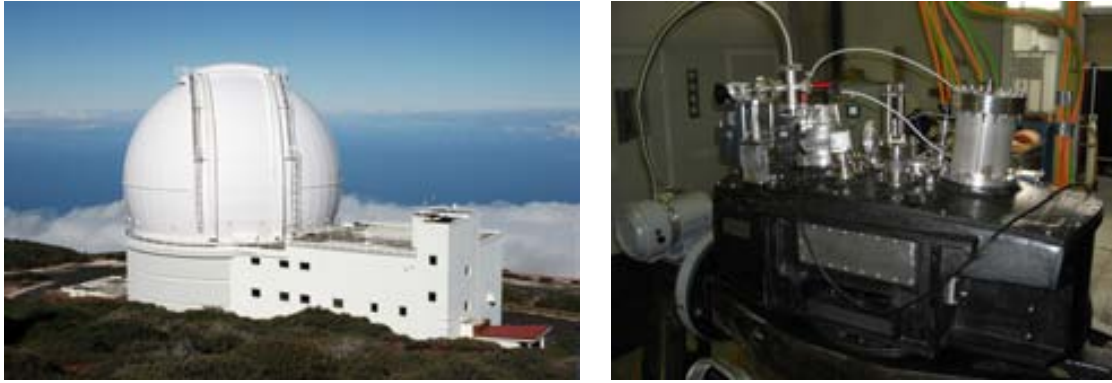
Figure 2.17: The William Herschel Telescope (WHT) dome (left) which will shelter PAUCam (right) whose photometric system is composed of 40 narrow bands.
