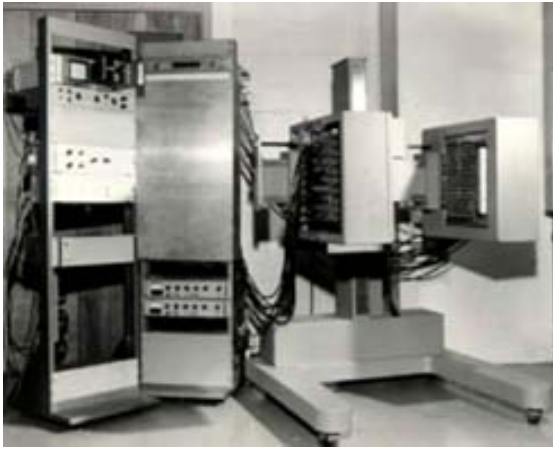
FIGURE 4.2: PC-I, the first tomographic PET imaging device. The figure is taken from [73].
