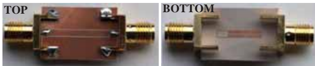
Fig. 5. Fabricated symmetric base CPW loaded with a folded SIR to validate the sensing principle. The substrate is the Rogers RO3010 with \epsilon_r=10.2 , h=0.127 mm, and \tan\delta=0.0023 . CPW dimensions are: L_{CPW}=20 mm, W=1.66 mm, and G=0.2 mm; SIR dimensions are: W_1=9 mm, W_2=0.2 mm, S=0.2 mm, l_1=12 mm, and l_2=2 mm.
