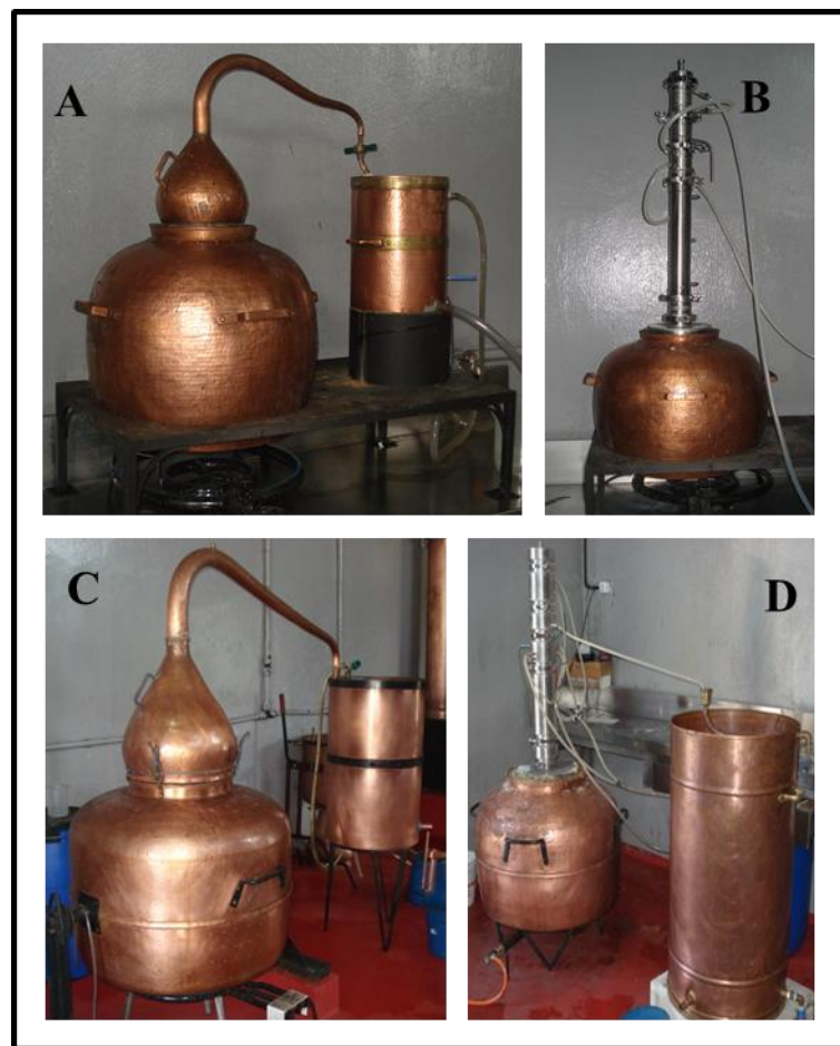
Figure 2.1. Distillation equipment used in this thesis. (A) 50 L-alembic charentais, (B) 50 L-packed column. (C) 300 L-alembic charentais, (D) 300 L-packed column.
