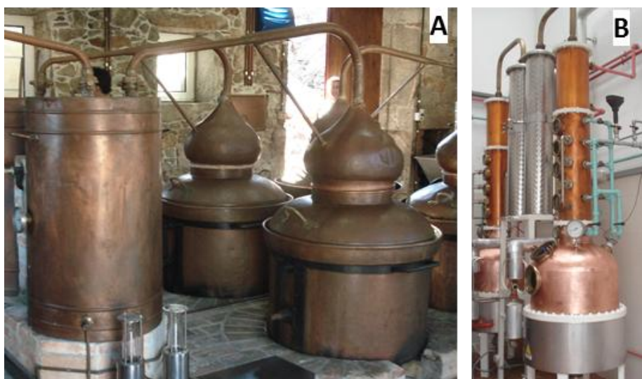
Figure 1.1. Distillation equipment employed in fruit spirits. (A) copper alembic, (B) distillation column (Holstein type).
