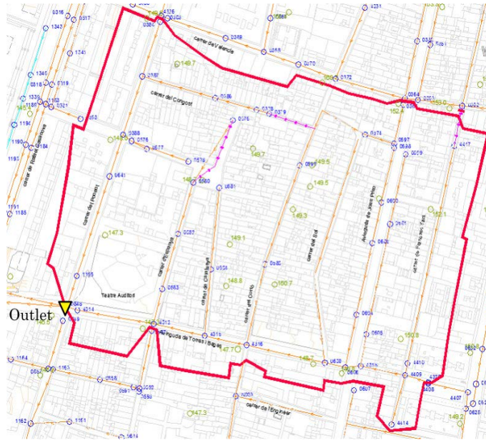
Figure 5-5 Partial image of the studied area obtained from a CAD file with the detailed data of the sewer network, street, site plan and topography information.
