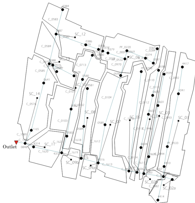
Figure 5-6 Layout of the combined sewer network implemented in SWMM5 showing manhole locations and catchment subdivision for the hydrodynamic modelling.
