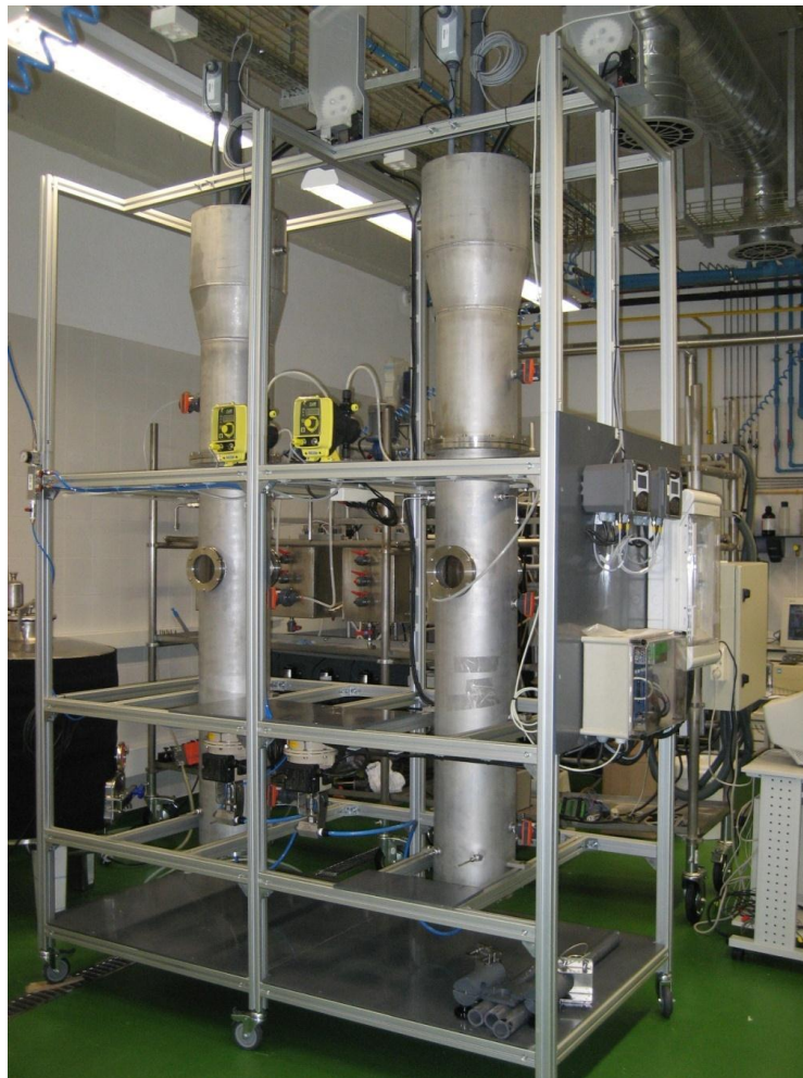
Figure 3.1. Picture of the GSB pilot plant for the treatment of a low-strength wastewater.
