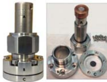
Figure 2.6. Electrochemical cell used for in situ X-ray diffraction measurements constituted by three main parts. A) Stainless steel plunger with a Be on the top where Na metal is placed. B) Body of the cell covered with a Mylar to isolate it from the plunger. C) Counter electrode current collector with Be window, where the active material to test is placed in contact with the separator.
