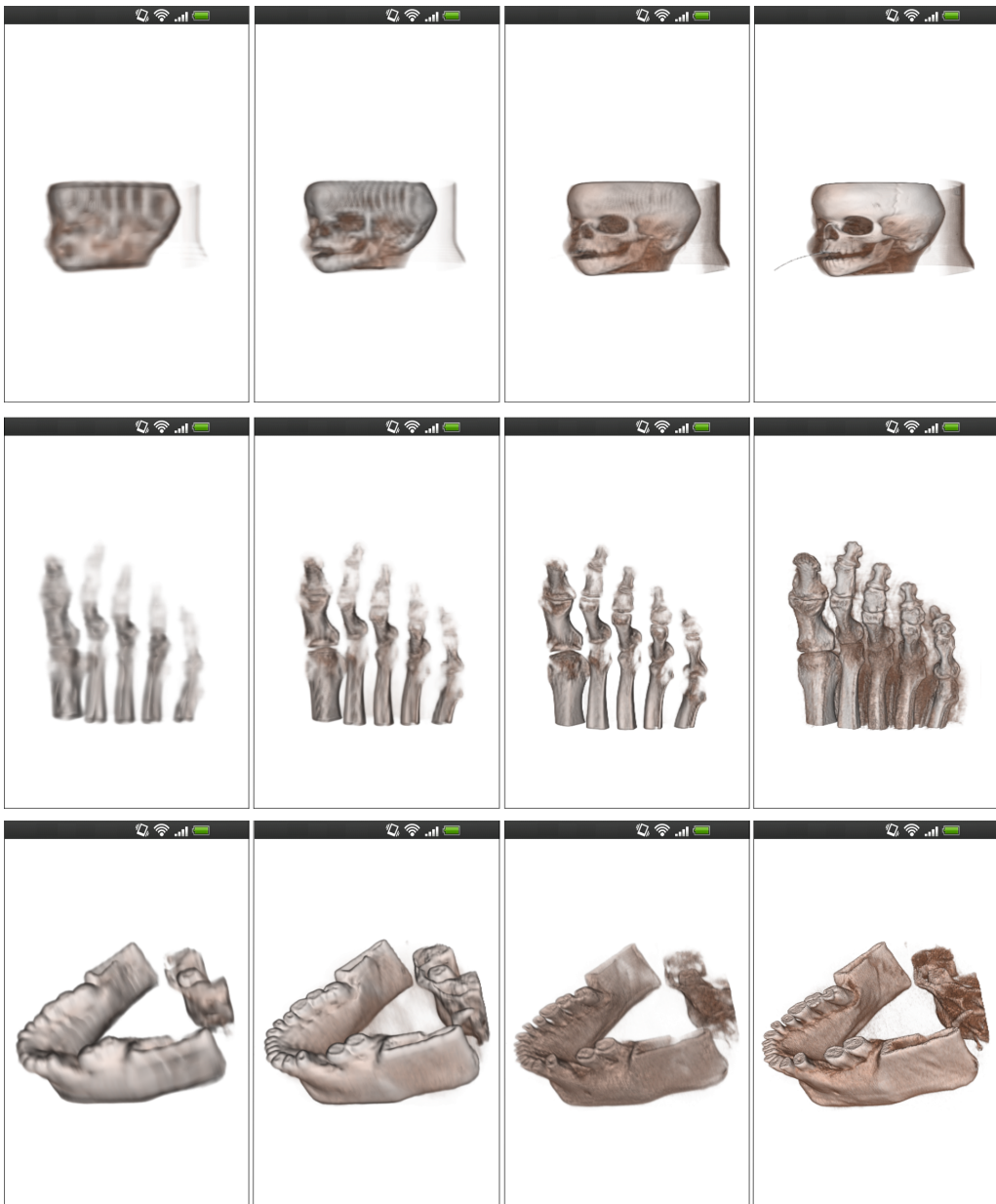
Figure 3.23: Rendering of the Skull, Foot and Jaw models in the HTC One Smartphone. The four columns show these models with Phong illumination and after applying one, two, three and four Wavelet reconstruction steps, from left to right respectively.
