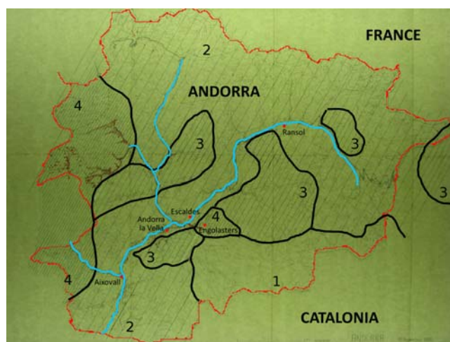
Fig. 5. Map reproduction of Andorra zoning of rainfall intensity estimation resulting from the terrain analysis made in December 1982. Four categories are considered: (1) Normal rain: no significant terrain movement; (2) Moderate rain: strong current marks, overflows, some traces of gullies, but almost no mark resumption of erosion and accumulation; (3) Heavy precipitation: important but not catastrophic marks; (4) Extreme precipitation: catastrophic marks. Different locations mentioned in the text are shown. Adapted from Barthélemy (1982).
