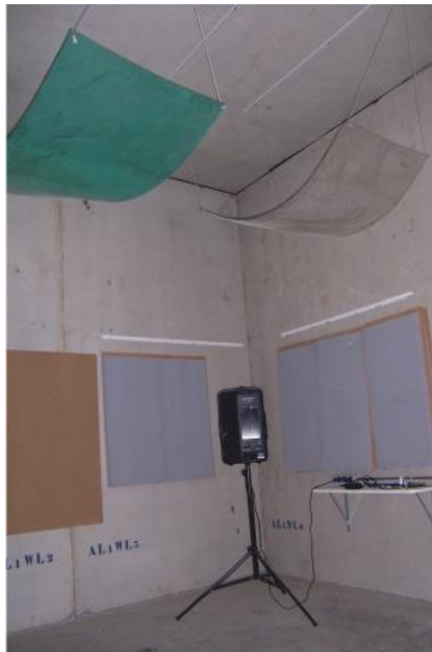
Img.C.5 Loudspeaker in the corner of the emission room during the testing (D)
