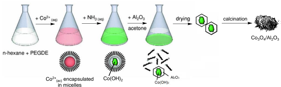
Figure 11. Schematic representation of the preparation of supported cobalt catalyst by microemulsion-destabilization. [84]
