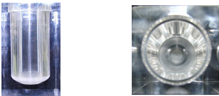
Figure 2. PMMA model of the vessel: lateral view (left) and top view (right)
