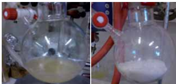
Figure 4.7. Gel formed from 46 and TEOS (left) and final hybrid silica material M11 (right).
