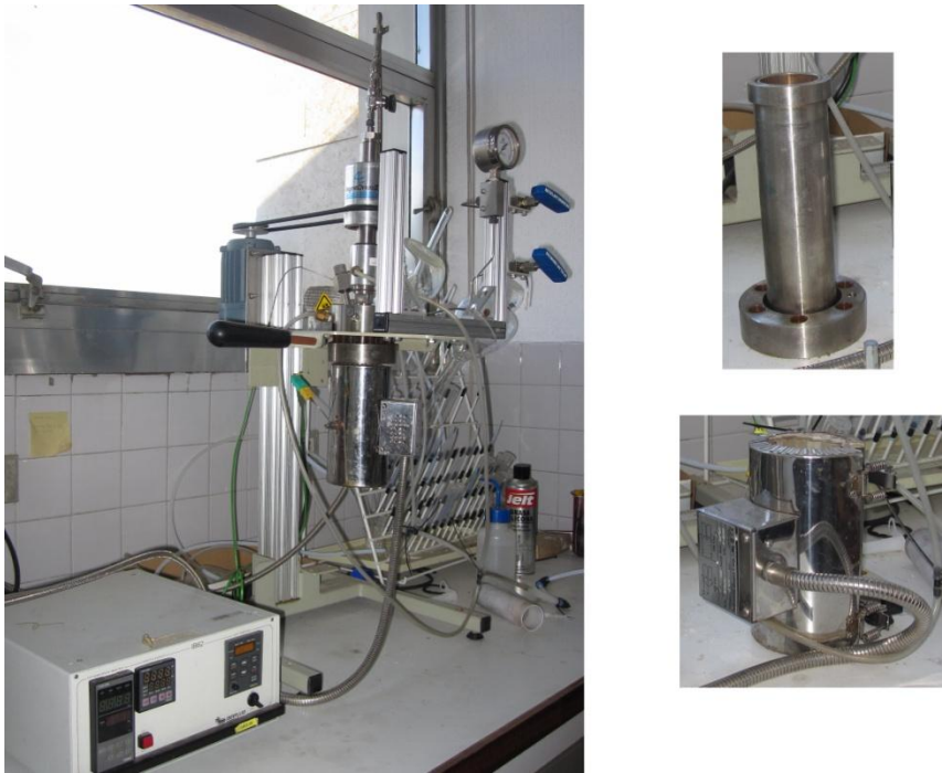
Figure 4.4. Low-temperature thermal treatment experimental device.
