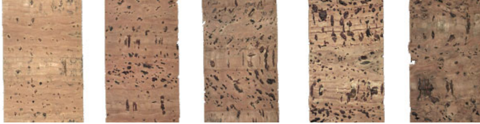
Figure 3.13: Cork stoppers of 5 quality groups ordered from best to worst quality (from left to right).
