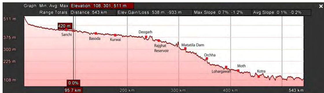
Fig. 2.7: Longitudinal Profile of the Betwa River
