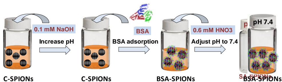
Figure 2. A schematic illustration of the pH adjusted and BSA adsorption protocol.
